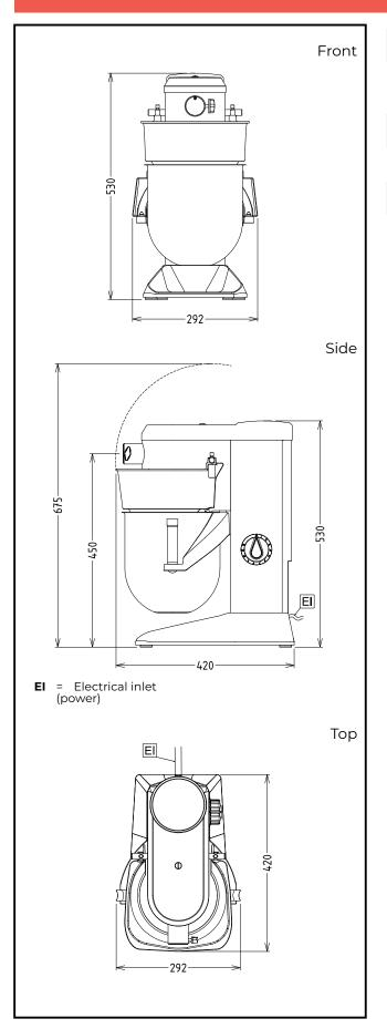
Electric Supply voltage: 200-240 V/1N ph/50/60 Hz **Electrical power max.:** 0.6 kW **Total Watts:** 0.6 kW Capacity: Performance (up to): 2.5 kg/Cycle Capacity: 8 litres Key Information: External dimensions, Width: 292 mm External dimensions, 416 mm Depth: External dimensions, Height: 527 mm **Shipping weight:** 20 kg Net weight (kg): 19 **Cold water paste:** 2.5 kg with Spiral hook
